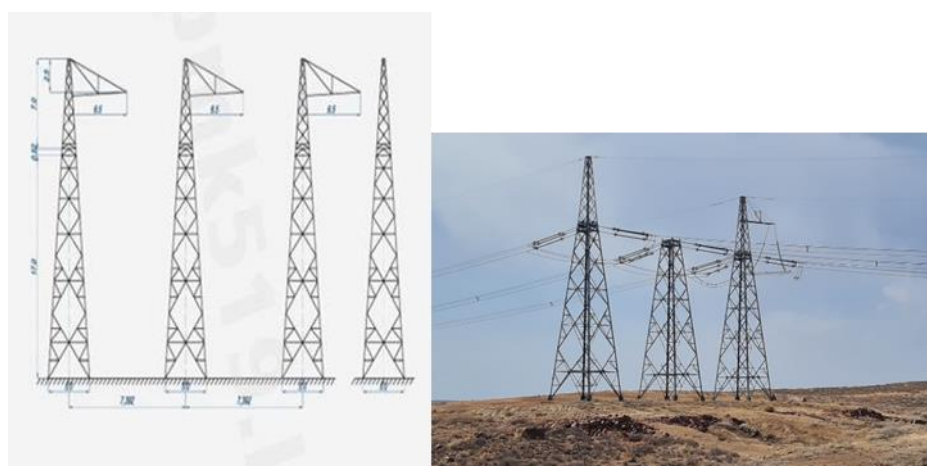
Figure 13: Structure n.3: Three-post lattice free-standing poles
